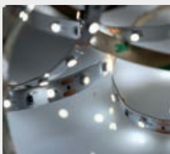
Standard Bright Cool White 6000K – 4.8W/m – 12V – IP20 Also available in 24V
